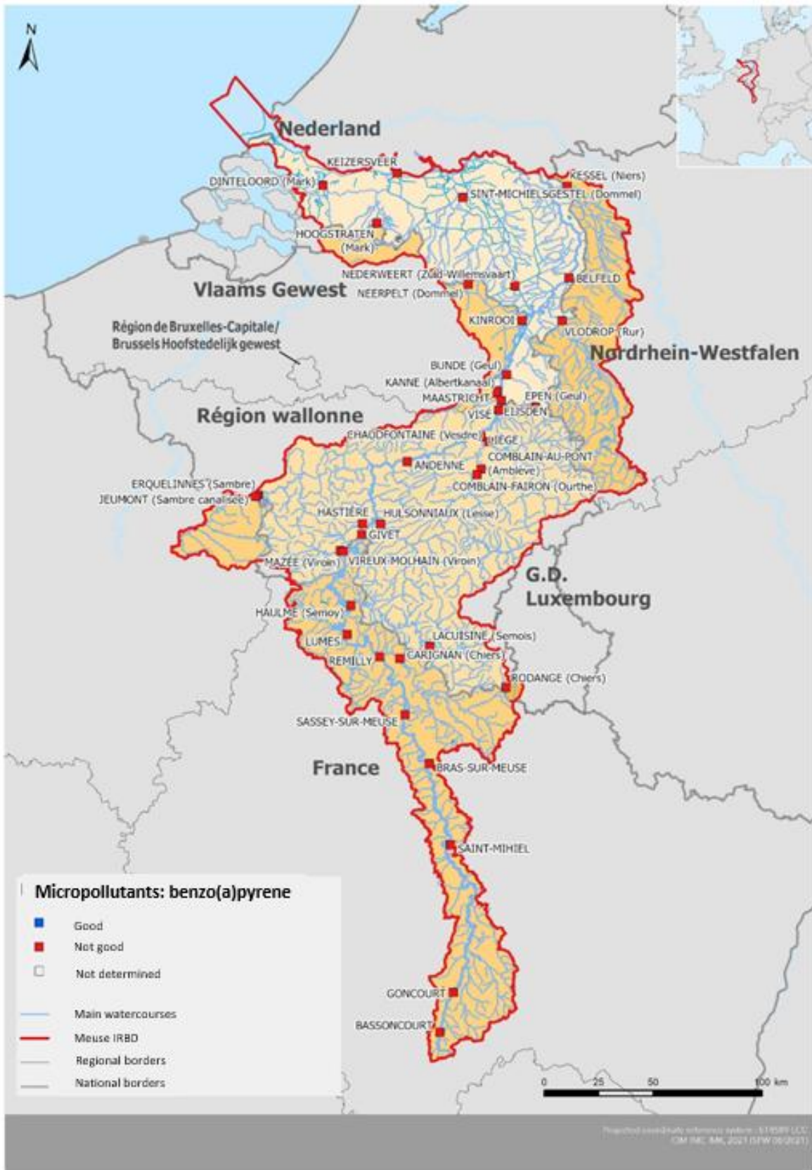
Map 4: Concordance with the EQS for the annual average concentration of benzo(a)pyrene in water at all HMR sites for the period 2017-2019
