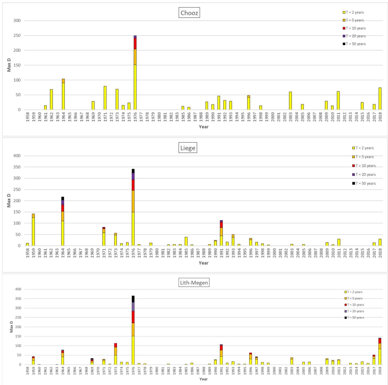
Figure 33: Maximum number of consecutive days in the year when the M7Q calculated for each calendar day was below a given threshold (MaxD parameter) for the return times of 2, 5, 10, 20 and 50 years - stations of Chooz, Liege and Lith-Megen (1958-2018)
